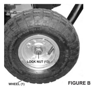
3. To attach the Wheels (1), slide a Wheel onto each end of the Axle located at the front of the Frame (2). Make sure air valve on wheel faces outward. Then secure the Wheels to the Axle, using one Lock Nut (13) for each Wheel. (See Figure B.)
